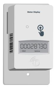
The Tehama Wireless Display MDT combines our proven MDT transceiver with a remote LCD display to provide the easiest and most accurate way to comply with tenant meter access requirements in California and elsewhere. The Display MDT is installed in the tenant space and wired to the remote meter. The LCD screen displays the consumption for 60 seconds when the button is pushed.
