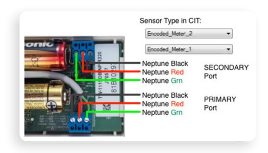
Note that you can swap the Meter connectors and the wiring order remains correct.
